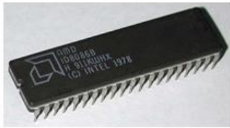
AMD ID8086B 5 MHz, 40-pin ceramic DIP
