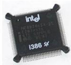
Intel NG80386SX-25 25 MHz, 100-pin plastic QFP
